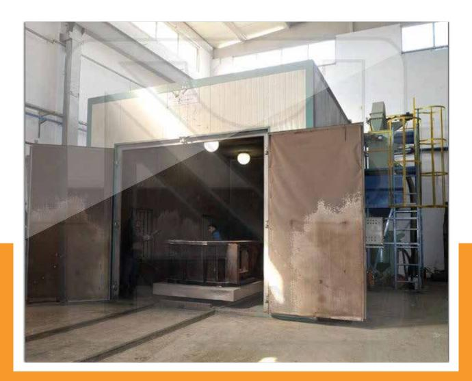
Our facilities include a dedicated steel ball cleaning operation with dimensions of  $4000 \times 5000 \times 8000$  mm. This state-of-the-art cleaning facility is equipped to handle large-scale works prepared for painting. Utilizing a ball spray system, we effectively address oxidation that may arise following the heat treatment process. In addition, our operations feature three specialized ball cleaning cabinets, each measuring  $1350 \times 1450 \times 1450$
