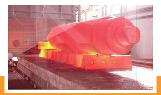
"Our facility includes an annealing furnace with dimensions of 2 meters in length, 2 meters in width, 2.5 meters in height, and a heating capacity capable of reaching temperatures up to 1250°C. This furnace operates on natural gas and is equipped with advanced features, including graphic measurement and drawing capabilities."
