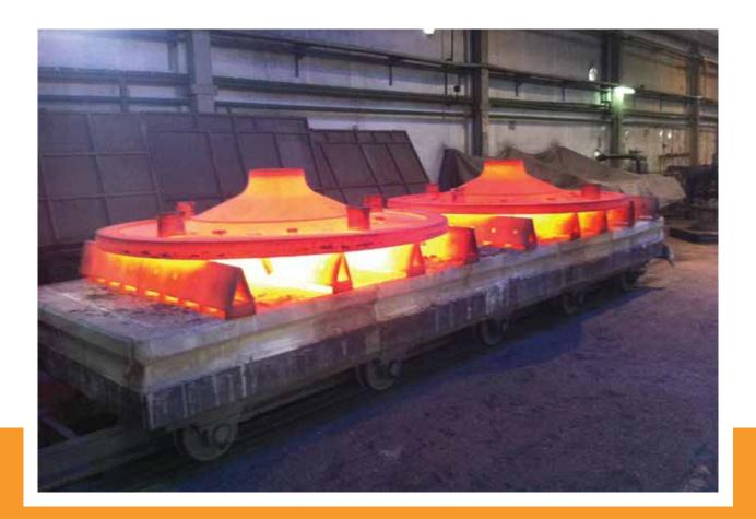
"We operate a well-type electric furnace measuring 1.5 meters in diameter and 3 meters in length, along with another well-type facility of the same dimensions. Our operations encompass natural gas reclamation, tempering, stress relief, and normalization processes. In addition to these facilities, we possess a 6-ton well-type oil tank and a water tank."
